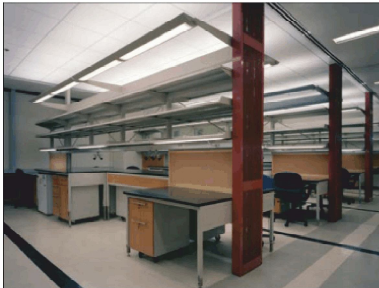
Figure 4: Mock-up of a lab module for Memorial Sloan Kettering Cancer Center, showing bench-mounted ambient lighting with under-cabinet task lighting. Source: ZGF Architects.
